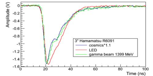
Comparison of pulse shapes induced by cosmic muons, LED pulses and gamma beam.
