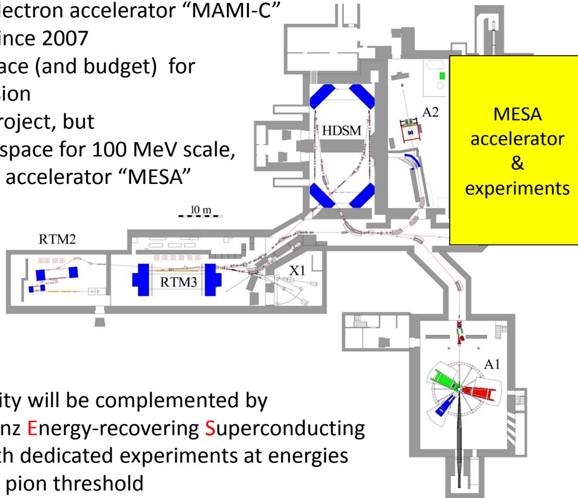
The MAMI facility will be complemented by **MESA**, the **M**ainz **E**nergy-recovering **S**uperconducting **A**ccelerator, with dedicated experiments at energies below or at the pion threshold
