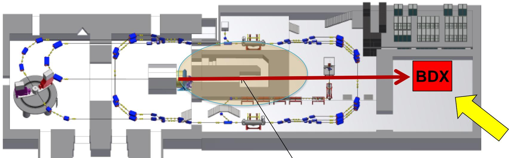
This existing beam dump is going to be the P2 beam dump
