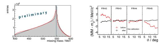
**Figure 2.** Left: Missing mass spectrum before (red line) and after the fine calibration (shaded filled area). Right: Deviation of the missing mass peak position depending on the polar scattering angle before (red line) and after (black line) the fine calibration.
