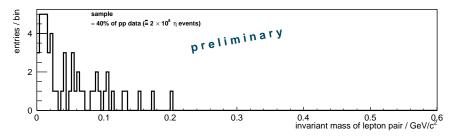
Figure 3. Invariant mass spectrum of the lepton pair after all cuts.
