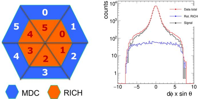
**Figure 2.** Left, schematic view of the rotation technique. Right,  $\Delta\phi$  (difference between  $\phi$  angle of the reconstructed track and  $\phi$  angle of the reconstructed ring)  $\sin\theta$
