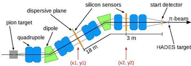
**Figure 1.** Schematic view of the pion beam line.
