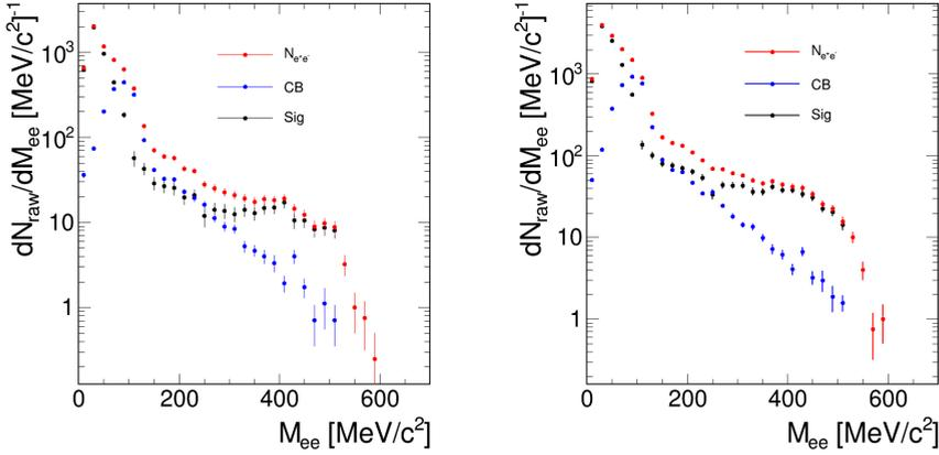
**Figure 3.** Raw inclusive invariant mass spectra using: left ring finder and right backtracking. Red solid circles show all  $e^+e^-$  combinations, blue solid circles show CB estimated using geometrical mean of same-event like-sign pairs, black solid circles show signal  $\text{Sig} = N_{e^+e^-} - \text{CB}$ .
