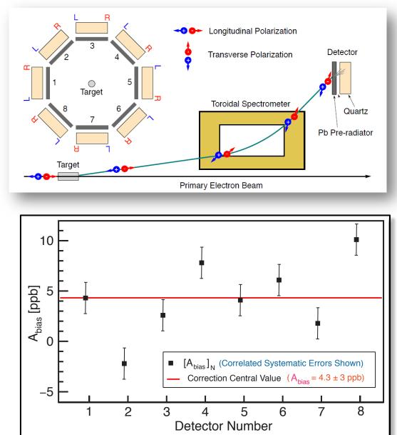
Saw a large, consistent asymmetry  $A_{diff} = (A_R - A_L) \sim 290$  ppb in the L & R PMTs of each detector bar.
