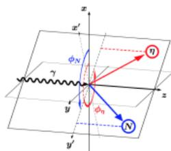
meson candidate (red) and recoil nucleon (blue) lie in the reaction plane, separated by azi.  $\delta\phi = 180^\circ$
