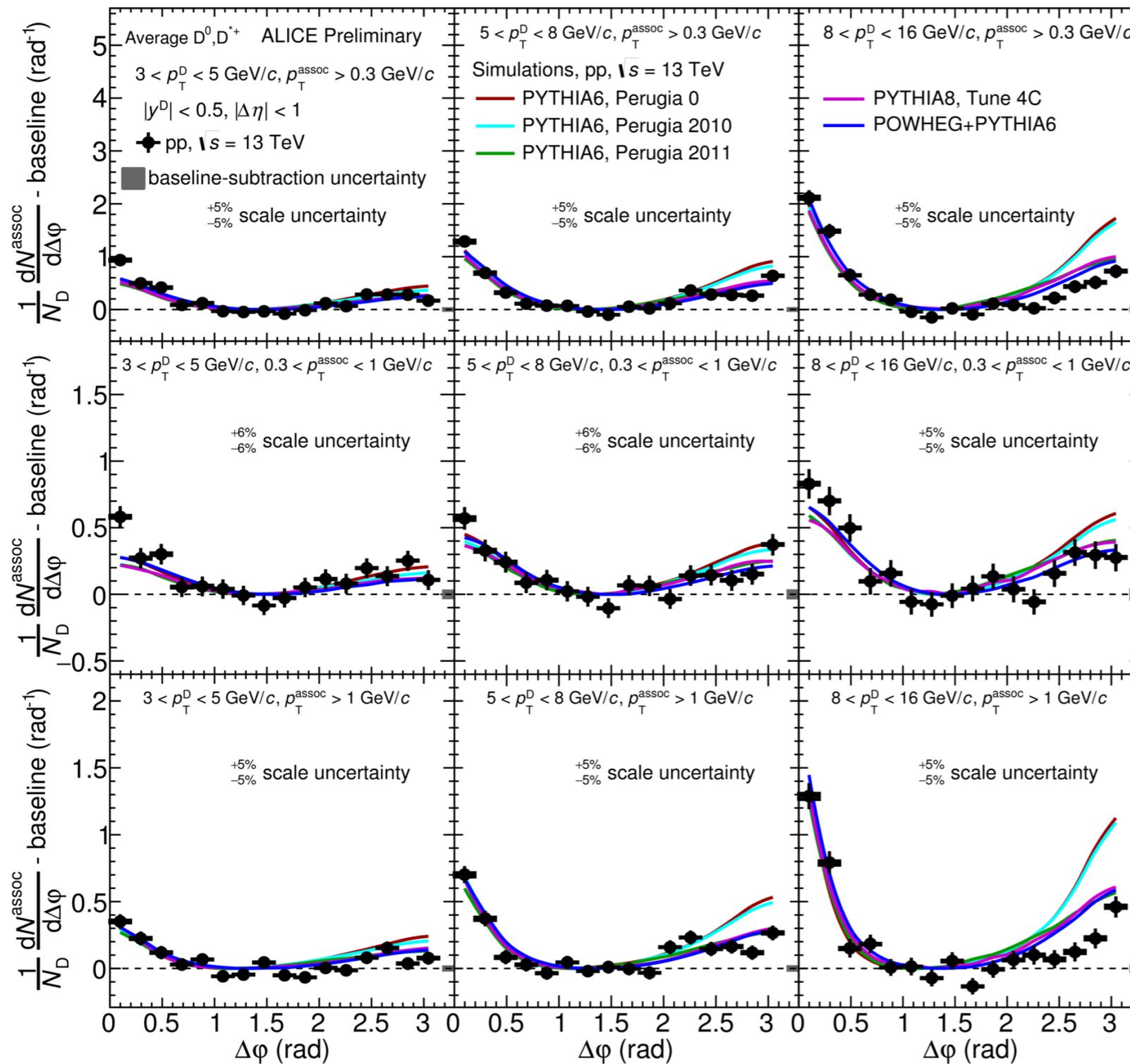
Comparison of  $\Delta\varphi$  correlation distributions in pp collisions and with expectations from Monte-Carlo simulations performed with different event generators, after the baseline subtraction.
